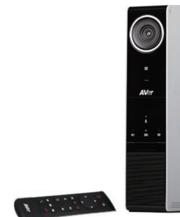
VC320 Conference Camera has a built-in camera, microphone, and speaker.
