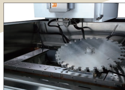
Equipped with a linear motor to eliminate backlash.
