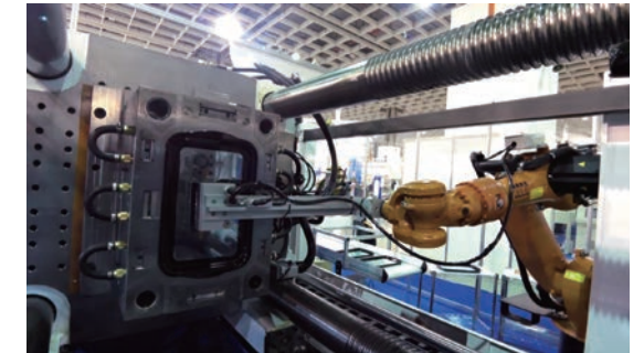
The melted plastic is injected from a long nozzle into the molds, which are installed on the side of the cube.
