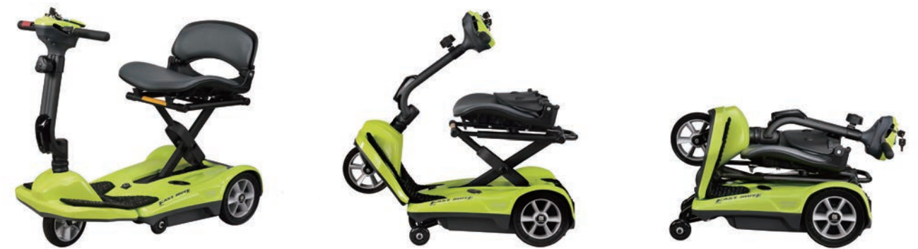
An electric mobility scooter which automatically folds when the button is pressed (Taiwan Excellence Silver Award received in 2017).
