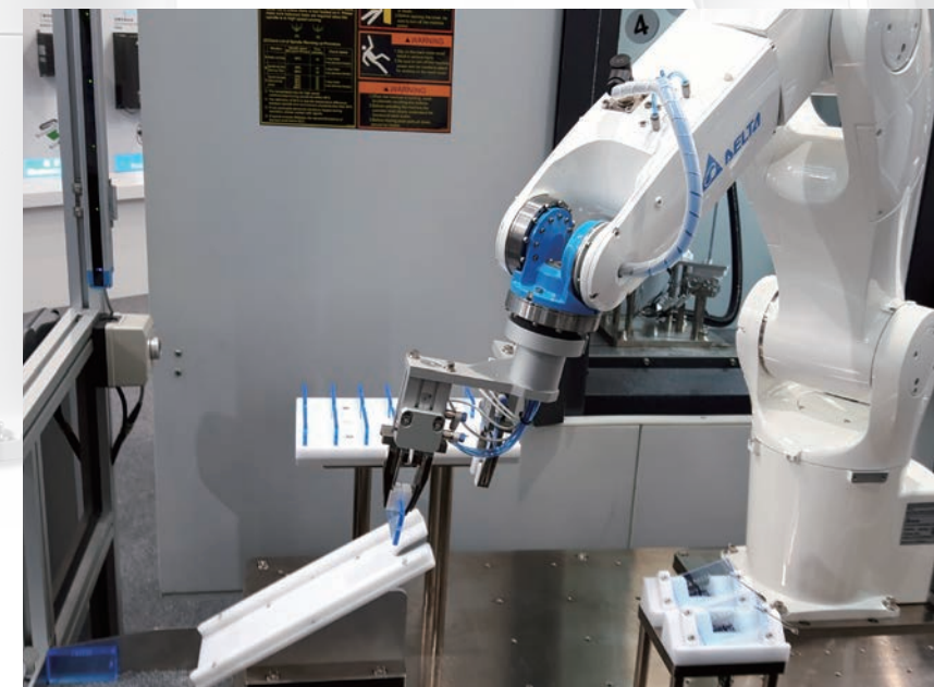
At the 26th Taipei International Machine Tool Show (TIMTOS), Delta Electronics articulated robot workstation, integrated with a CNC machine, MES (Manufacturing Execution System) and cloud, produces customized gifts on site.
