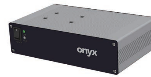
The small desktop personal computer "MedPC-2100" for medical institutes does not need a cooling fan.
